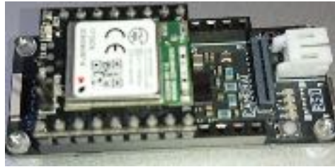
Connection between WiFi Addon and Spresense MainBoard
